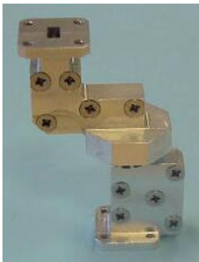
**Figure 6: Waveguide rotary joint incorporating two E-plane probe transitions**
