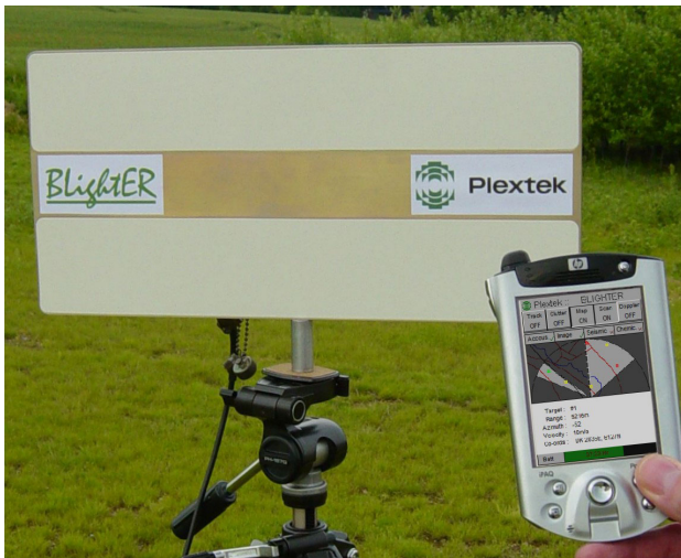
Fig. 1. The radar consists of a single portable unit containing all elements of the FMCW radar. A standard wireless link provides a low cost interface to a laptop or PDA (shown).
