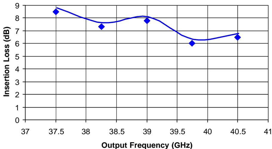
**Figure 13: Measured conversion loss of frequency trebler versus output frequency**
