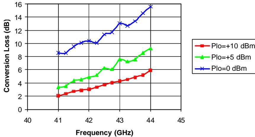
**Figure 11: Measured conversion loss at various LO power levels**
