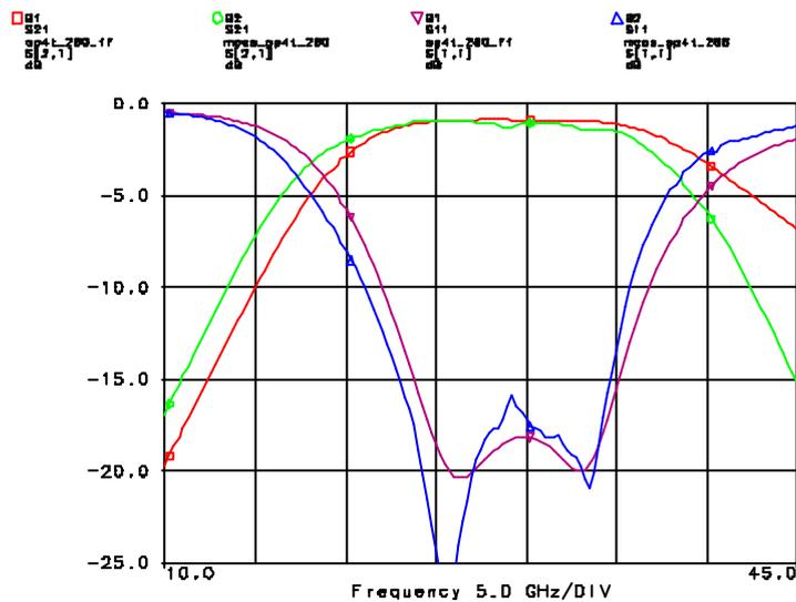
Figure 17: Measured versus simulated small-signal performance of one branch of the low-band SP4T MMIC in the on state
