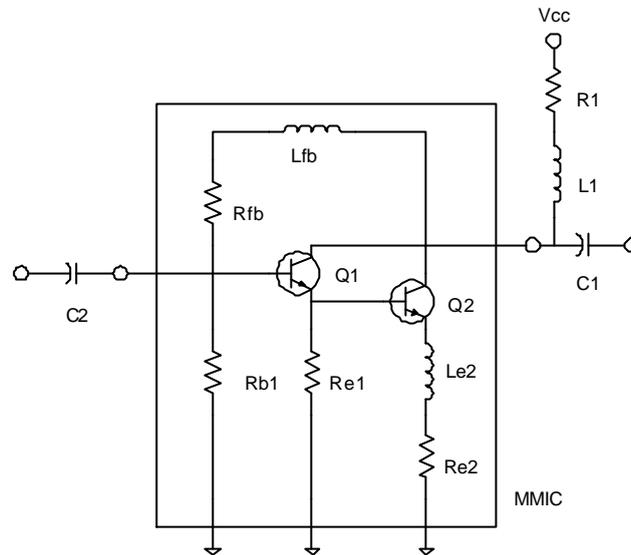
**Figure 5: Simplified schematic for the broadband Darlington pair amplifier**
