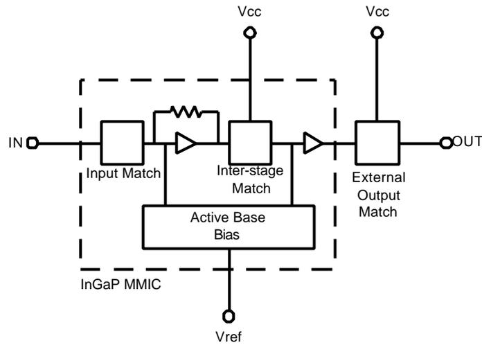
**Figure 2: Simplified schematic of the U-NII PA**
