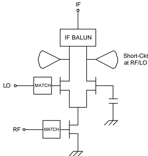
**Figure 9: Simplified schematic of the mm-wave Gilbert-cell mixer**
