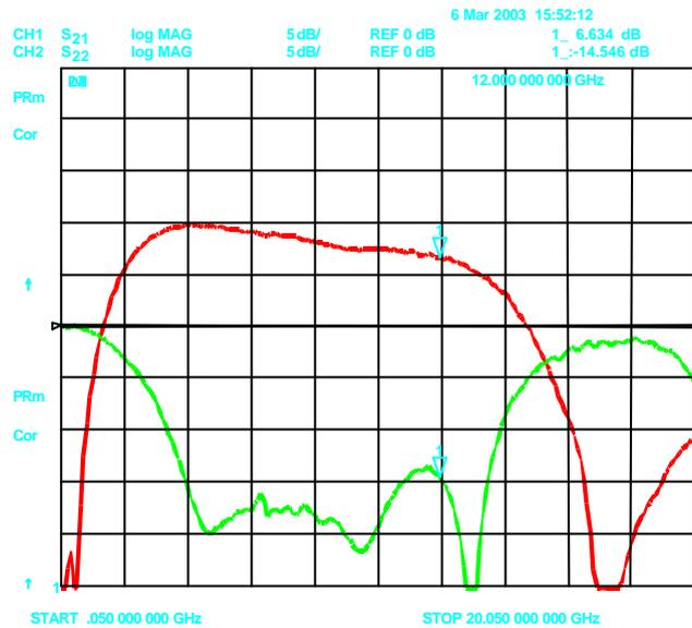
**Figure 7: Measured small-signal response of broadband amplifier with external matching**
