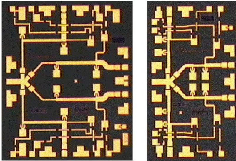
Figure 16: Photograph of the SP4T MMICs (24 to 34GHz design on the left, 34 to 45GHz on the right)
