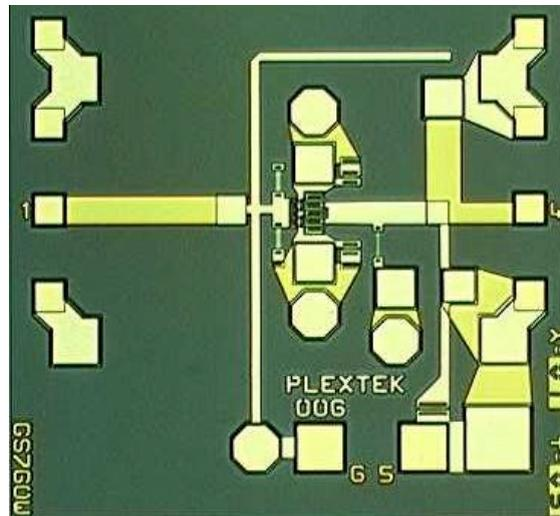
**Figure 12: Photograph of the pHEMT MMIC trebler**
