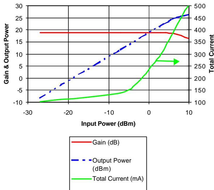
**Figure 4: Measured performance of the U-NII PA versus input power**
