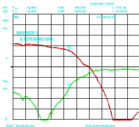
**Figure 6: Measured small-signal response of broadband amplifier without external matching**
