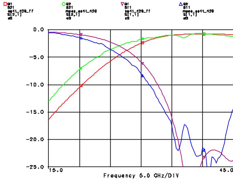
**Figure 18: Measured versus simulated small-signal performance of one branch of the high-band SP4T MMIC in the on state**
