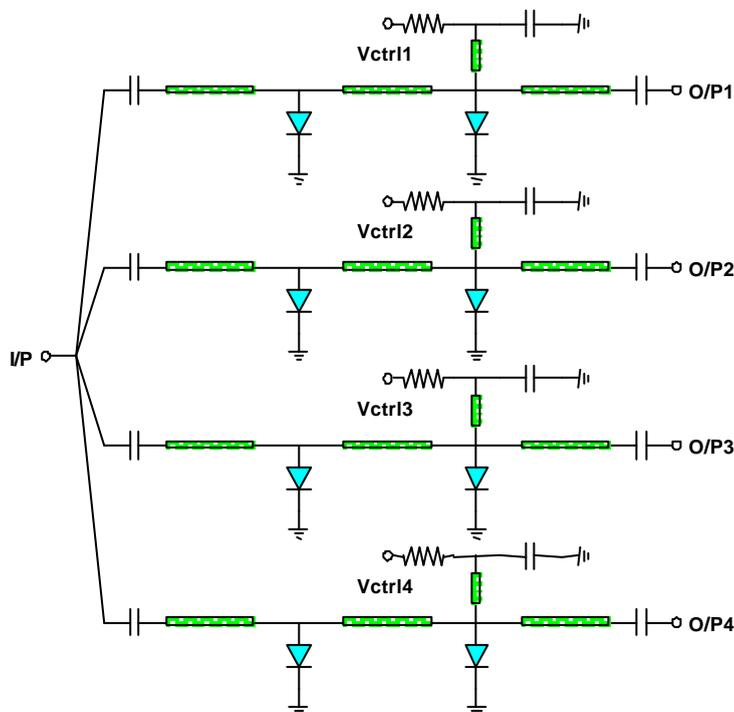
**Figure 15: SP4T switch schematic**
