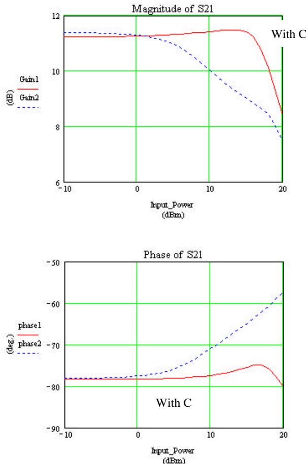
**Figure 3: Effect of linearising capacitors on the magnitude and phase of the gain**
