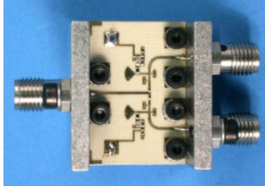
**Figure 11: Photograph of SPDT in test jig**
